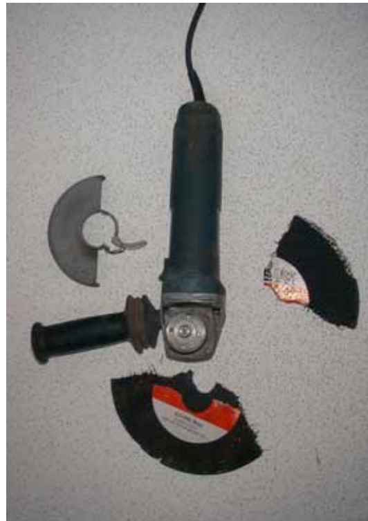
Angle grinder and disintegrated disk
